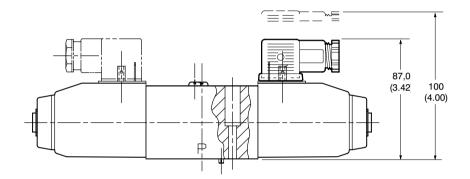
Connector can be positioned at  $90^{\circ}$ intervals on valve by re-assembling contact holder into appropriate position inside connector housing.
