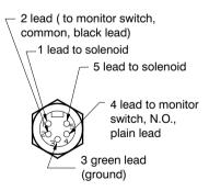
▲ Electrical connection is over solenoid on single solenoid models, and over "b" solenoid on dual solenoid models. See diagram plate for "b" solenoid location. Electrical rating 600 volts, 3 pole, 10 amps and 5 pole, 8 amps. The female portable plug to be furnished by customer.
