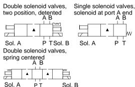
solenoid at port A end A B ٨٨ P Т ΡТ
