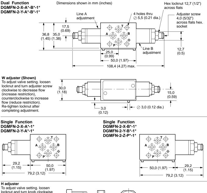
locknut and turn knob clockwise to decrease flow (increase restriction), counterclockwise to increase flow (reduce restriction). Re-tighten locknut after completing adjustment. **K adjuster**
