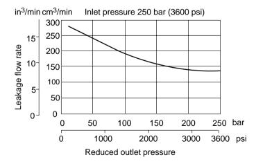
Note that the effective reduced pressure is the sum of the valve adjustment and any back pressure in line T. The effect is illustrated below.
