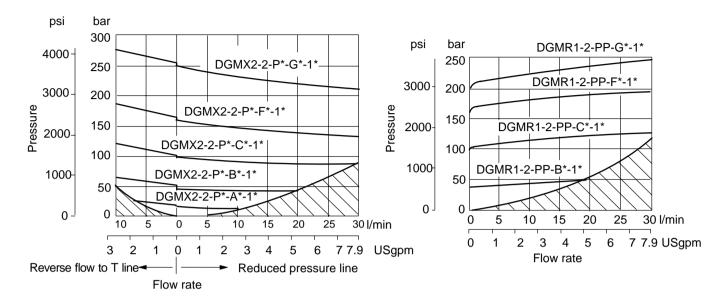
Note: Valves will not function at pressure/flow values in shaded area.
