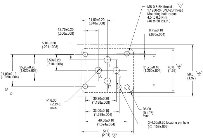
The minimum thread depth is 1.5 of bolt diameter. The recommended full thread depth is 2xD+6mm to aid in the interchangeability of valves and to reduce the number of fixing bolt lengths. The recommended engagement of fixing bolt thread for ferrous mountings is 1.25 D.
